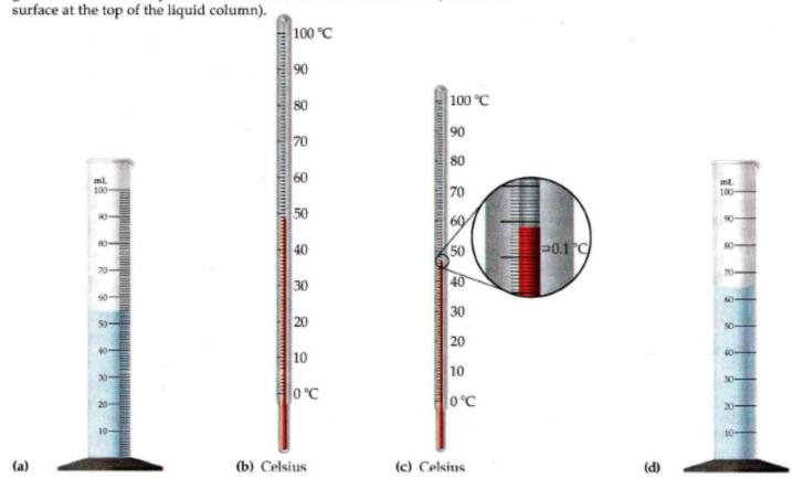
Read each instrument to the correct number of significant figures. Laboratory glassware should always be read from the bottom of the meniscus (the curved surface at the top of the liquid column).
